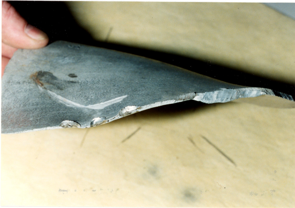
51. Another close-up view of the edge of the aluminum tank fragment
